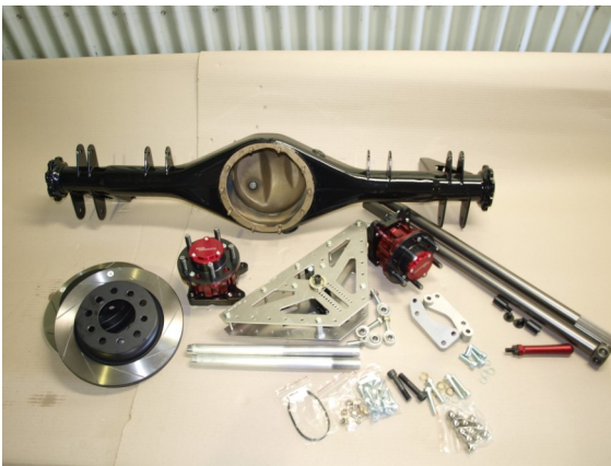
The freshly powder coated diff housing is laid out with all of the components required for the kit, everything is double checked prior to final assembly
