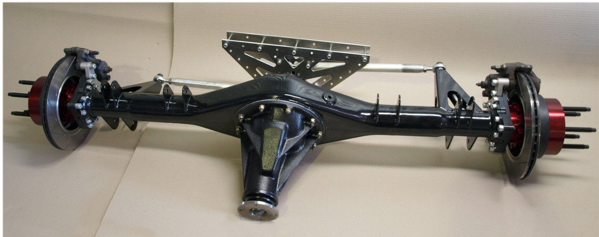
Fully Assembled, complete with one of our Watts Linkage Kits, Kaaz LSD Centre, Race Products Brake Kit, and custom wheel adaptors. We have many different options available, Please contact us for pricing to suit your car.
