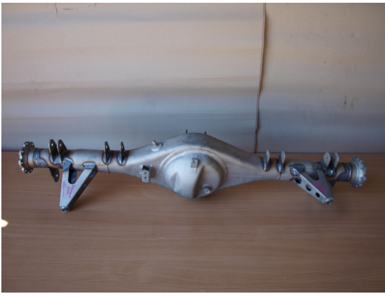
Fabrication completed, the housing is ready for re-finishing.
