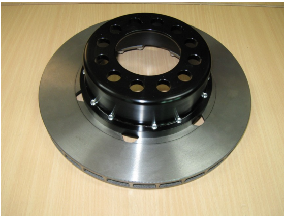
Our Floating Rotor Kits use a 278mm Diameter Rotor, sourced from a Formula 3 Car, coupled with a Disc Bell Made from Aircraft Grade Aluminium Billet
