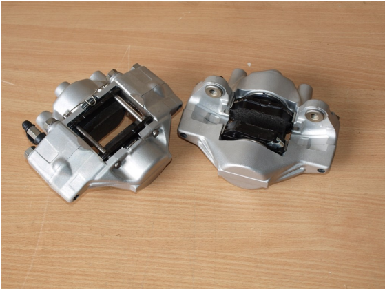
Our Standard Option for these kits is to use the Nissan 300ZX/Skyline Rear Caliper. These lightweight 2 piston calipers offer a powerful and cost effective solution for most customers.
